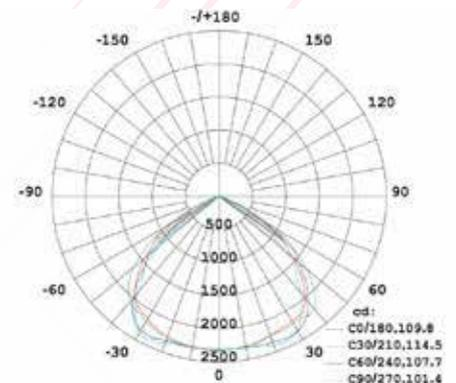
Beam spread diagram showing illuminance at a distance (Center Beam LUX) for various heights and diameters:
