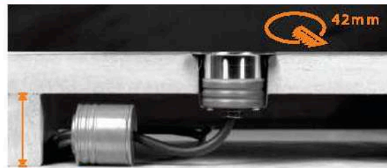
A: Minimum space for external driver is 48mm B: IP67 120V/240V/24V & RGB 24V external input driver
