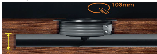
A: Minimum space for external driver is 20mm.
