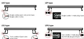
Low voltage input factory default: Double outlet - The power cord is in the form of LTO type Waterproof male and female plugs are optional . (Other power cable type and male and female plugs are optional)
